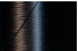
Galvorn fiber tow consisting of many individual fiber filaments. FIBER TOW
